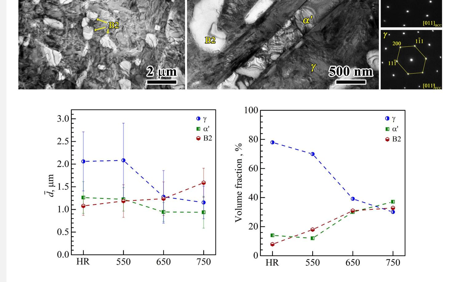
As the aging temperature increases, the volume fraction of  $\gamma$ decreases, whereas those of **B2** and  $\alpha$ ' increase simultaneously. However, the grain size of B2 increases overtly, which is detrimental to ductility since it is hardly deformed.
