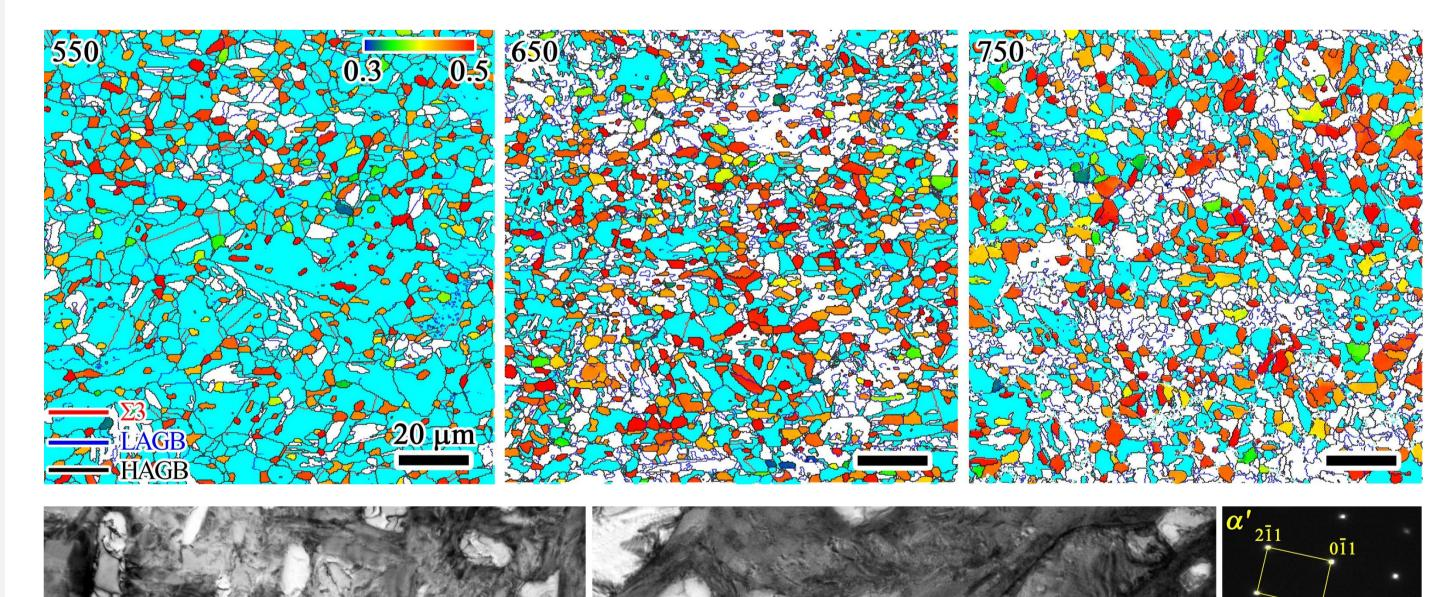
The martensite transformation of the retained austenite and highdensity martensitic twins can be observed in the aged samples after deformation, rendering a significant strain hardening.
