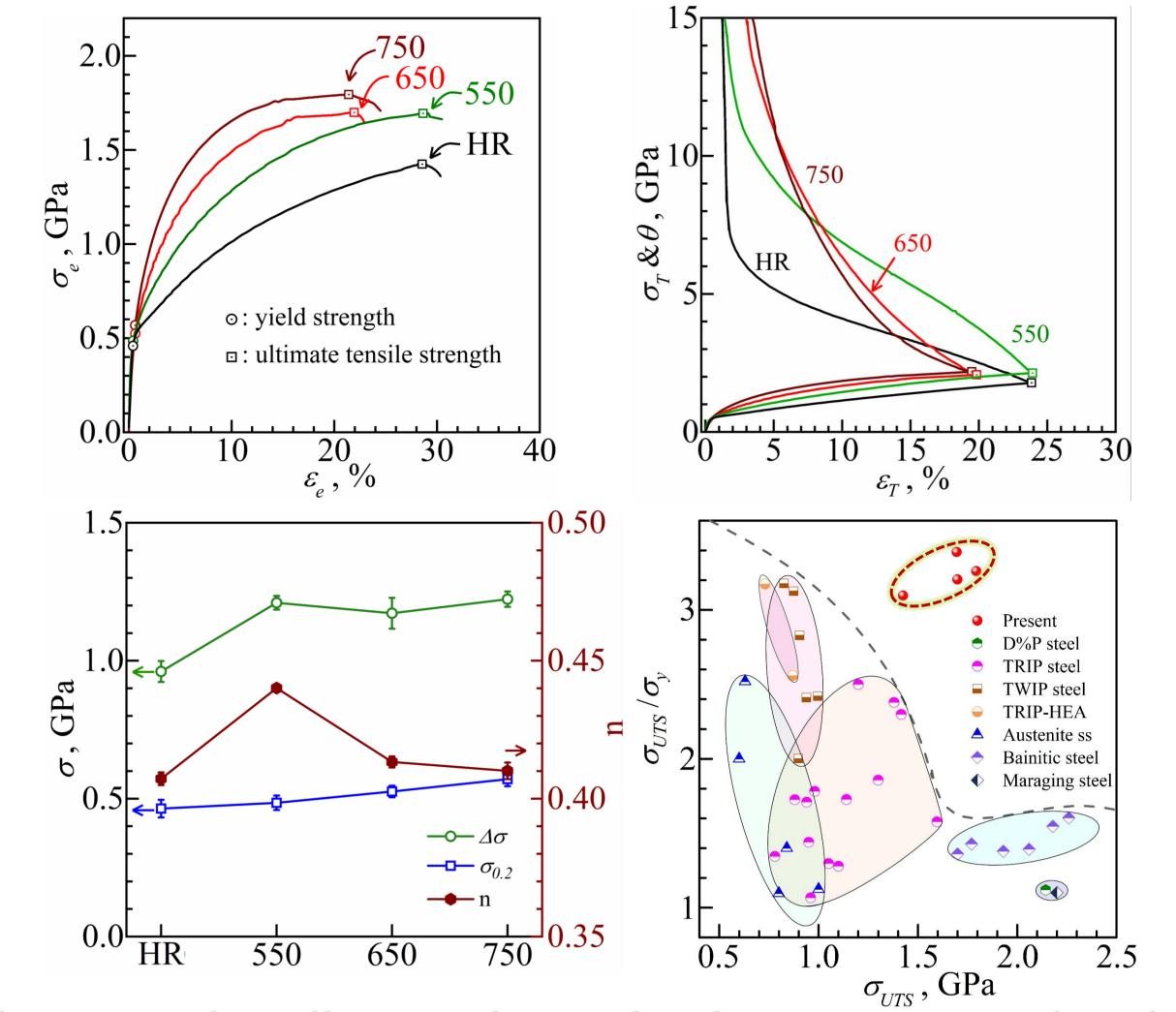
To this end, we report a strategy for achieving an extraordinary high strain hardening rate by introducing a triple-phase microstructure, containing the B2 precipitates and martensite for strengthening, and the retained austenite for the TRIP effect.
